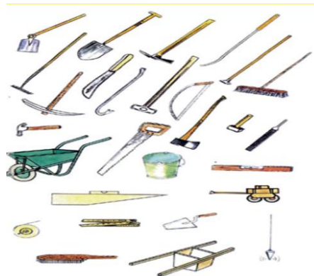
Figure D-1. Tools used for construction and maintenance of foot trails
